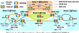
Figure 1. Configuration of multi-area MPLS/GMPLS interoperability testbed
