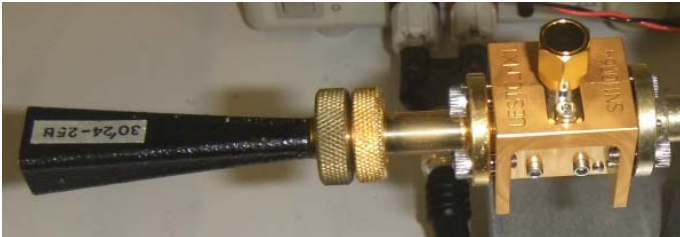
Fig. 4 Feed horn integrated 380GHz mixer
