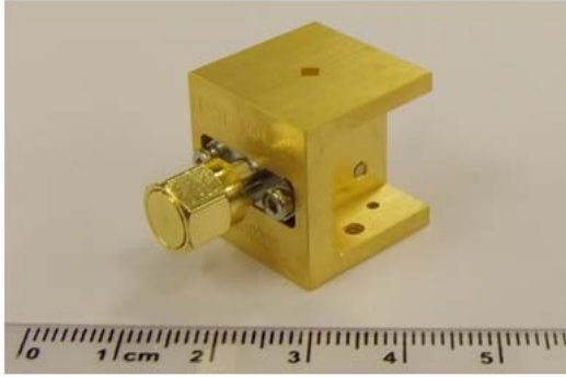
Fig. 8 The 380 GHz SHP mixer after assemble
