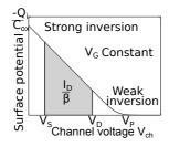
Figure 1: Drain current according to Eq. (4).
