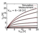
Figure 4:  $I_{DS}$ - $V_{DS}$  characteristics.
