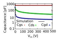
Figure 5: C-V<sub>DS</sub> characteristics.
