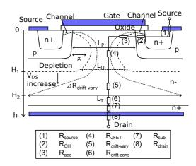
Figure 3: Cross section of the VDMOSFET with parasitic resistances.
