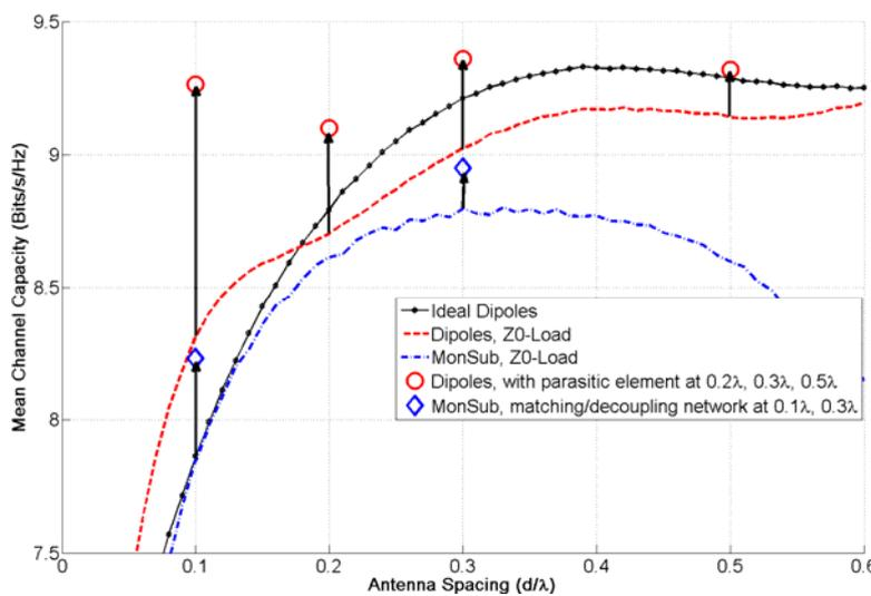
Figure 5: 2 x 2 MIMO-channel capacity for antennas with matching networks and/or parasitic elements for selected antenna distances on the receiver side.
