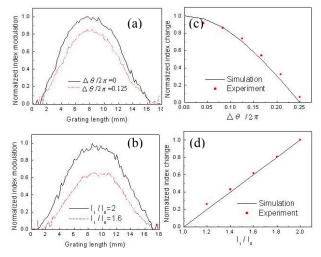
Fig. 2. (a)Index profiles of single grating section in configuration 1. (b)Index profiles in configuration 2. (c) Index modulation in configuration 1. (d) Index modulation in configuration 2.
