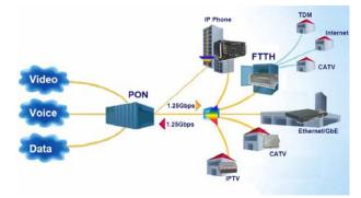
Fig.3. FTTH multi-services based on GEPON
