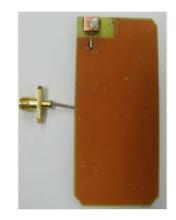
(a) Proposed antenna (b) Proposed antenna with PCB Figure 2: Fabricated antenna
