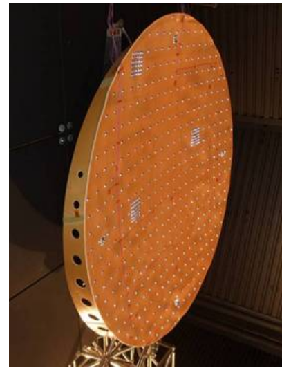
Fig.5 Manufactured dual gridded reflector (Diameter 2.2m)
