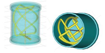
Fig. 3 3D simulation model of the quadrifilar helical antenna
