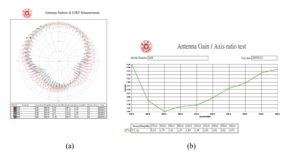
Fig. 6 (a) Measured radiation patterns, and (b) measured axial ratio vs. frequency
