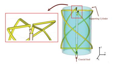
Fig. 2 Feeding structure of the present antenna
