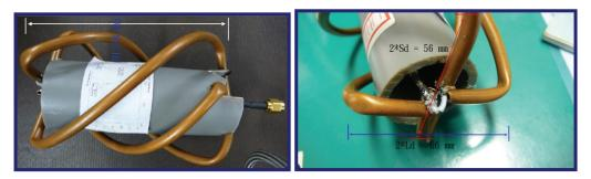
Fig. 1 Construction of the present quadrifilar helical antenna and its detailed dimensions
