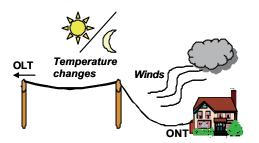
Figure 1: Schematics of FTTH and environmental effects
