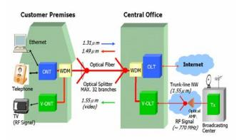
Fig. 1 Gigabit-Ethernet Passive Optical Network (GE-PON)
