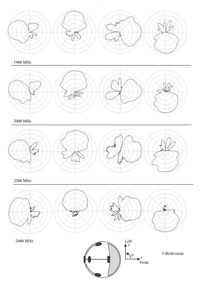
Figure 3. Measured azimuth patterns of breadboard model in four beam states over 1.9–2.4 GHz at  $\theta$  = 90°.
