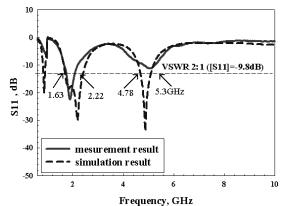
Fig. 2: S11 simulated and measured result for F-PIFA
