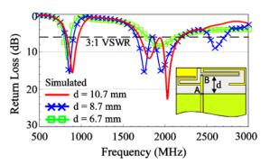
Figure 5: Simulated return loss for the proposed antenna as a function of the position dof the printed distributed inductor. Other dimensions are the same as given in Fig. 1.
