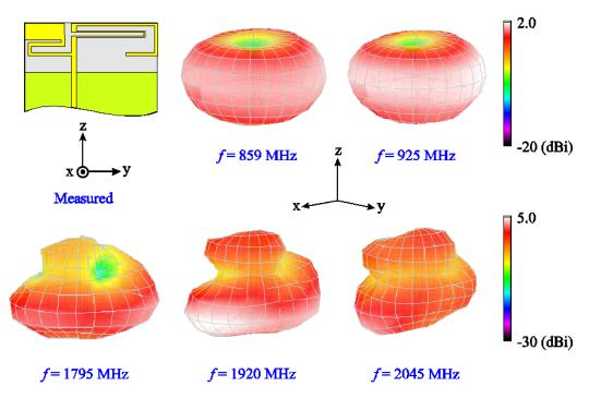
Figure 6: Measured 3-D radiation patterns for the proposed antenna.
