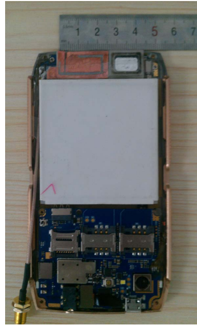
Fig 2. Fabricated penta-band mobile phone antenna
