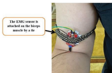
Fig. 4: shows how the tie was used to assure the fixed contact between the EMG sensor and the biceps muscle
