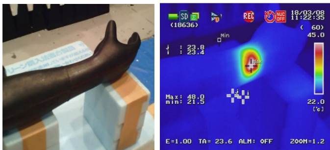
Fig. 8. Measured result of temperature rise after 60 sec. irradiation. (Antenna input power : 15 W, measured by infrared thermography)
