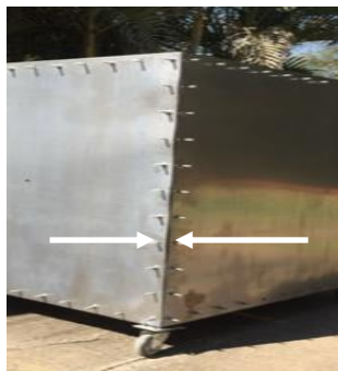
Fig. 4. Cubic structure (1×1 m) covered with metallic plates with small gaps in the edge joints used on the experiments (between white arrows).
