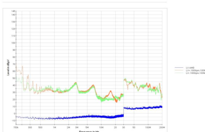
Figure12. CE results of LV ports with HV injection under one dynamic status
