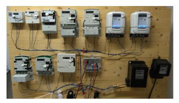
Fig. 1: Ten static meters placed in series.
