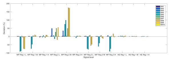
Fig. 4: Deviations [%] between the 10 static meters (SM) and reference, for different combinations of water pump (WP), heater (HE) and regulator (Reg).
