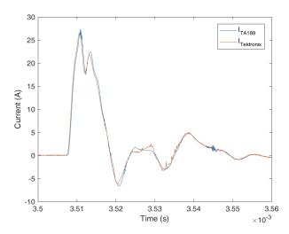
Fig. 2: Comparision between TA189 and Tektronix current probe, for a close-up of the line current as observed during the measurements.
