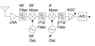
Figure 3 Block diagram of the Heterodyne Receiver.
