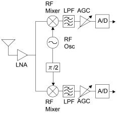
Figure 4 Block diagram of the Direct Conversion Receiver.
