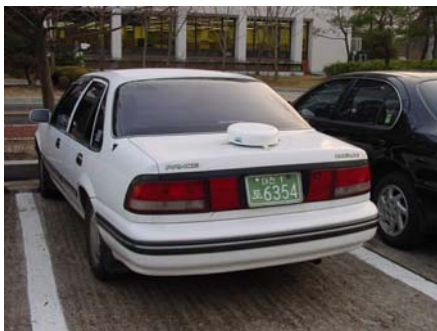
Fig. 8 Test antenna system installed on a car
