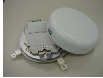
Fig. 4 Active phased array antenna system
