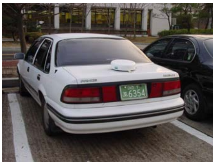
Fig. 8 Test antenna system installed on a car
