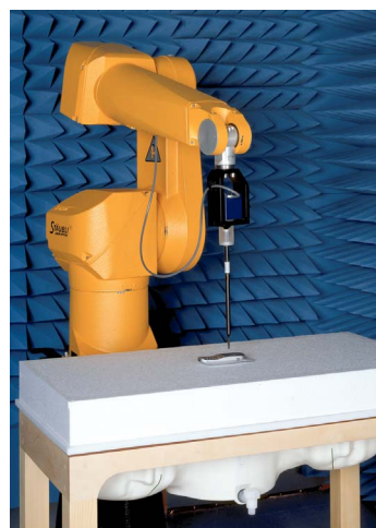
Figure 2: Dosimetric assessment system DASY4: free space measurement of mobile phone.
