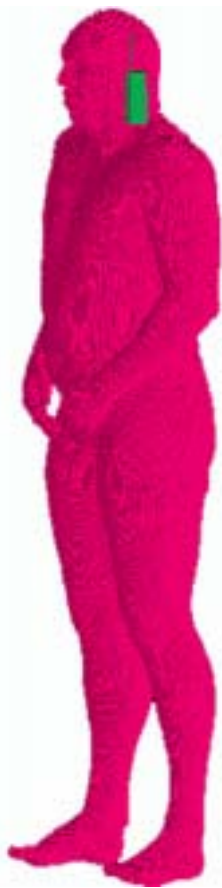
Fig.4 A visualization of the whole body human model together with a 900 MHz mobile phone model.
