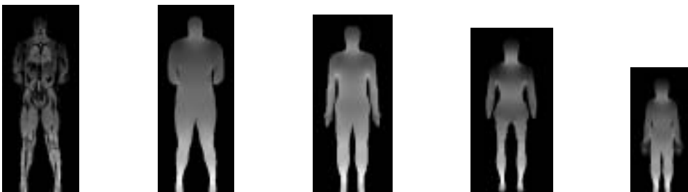
Figure 4: SAR distributions in the vertical section of the whole-body human models (inhomogeneous-tissue European-American (EA) adult male, homogeneous-tissue EA adult male, homogeneous-tissue Japanese adult male, female, and child) exposed to E-polarized TEM wave at 38 MHz. The SAR is normalized by the maximum value in the section and shown in logarithmic scale.
