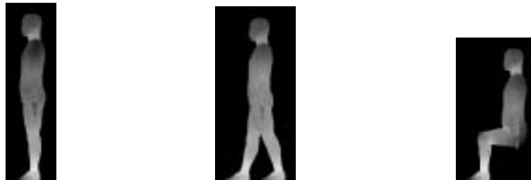
Figure 8: SAR distributions on the surface of the whole-body human models exposed to E-polarized TEM wave at 38 MHz.
