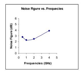
Fig. 5 Measured noise figure vs. Frequencies.
