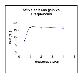
Fig. 4 Measured active antenna gain vs. Frequencies.
