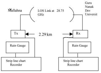
Fig.1 Experimental setup for rain attenuation Measurement
