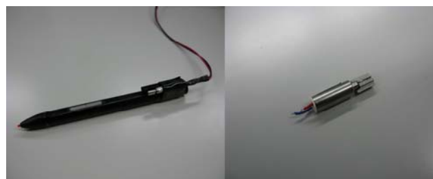
Figure 1. stylus with an attached motor and the motor
