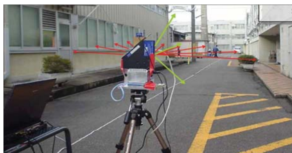
Fig. 3: Improvement of Spatial perception ability using Milliwave radar data, Stereo camera data and Gyroscope sensor data.
