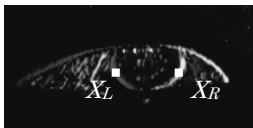
Fig. 8 Vertical edge detection with sobel filter.
