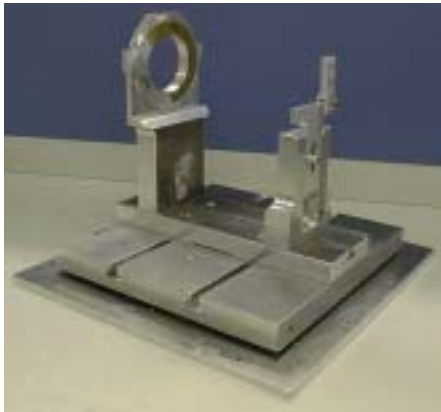
Fig.3 Special jig in the final stage
