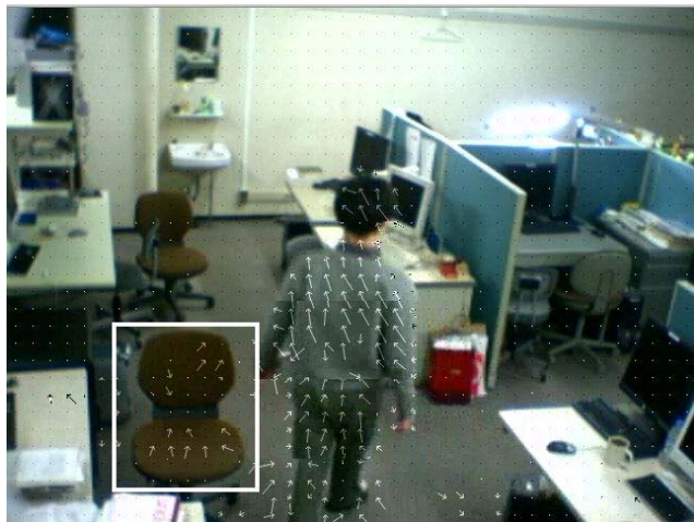
Figure 4: Motion vectors in an MPEG-2's P-frame
