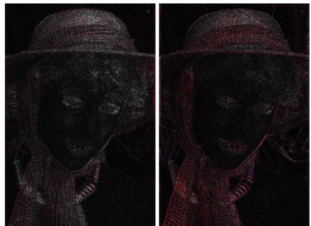
(a) The redundant DCT demosaicing (b) The Haar-wavelet demosaicing
