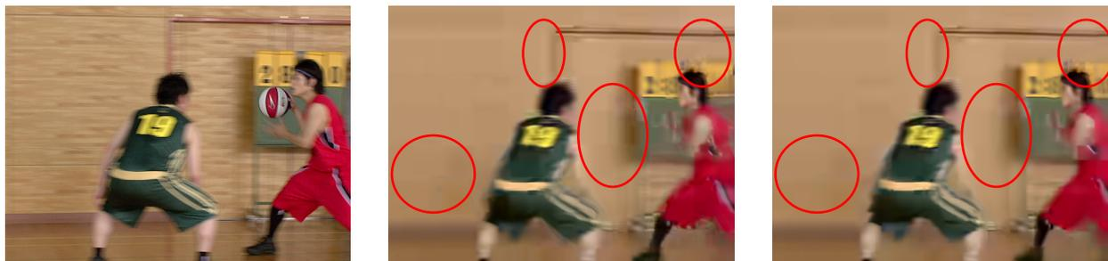
Fig. 2: Original and decoded images by the JEM2.0 and the proposed method. Red circles show significantly different area by the proposed deblocking filter.
