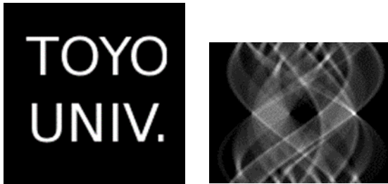
Fig. 3. The Original test image (128×128pixel, 8bpp) and its projection data (Sinogram: 128 Detectors, 100 Views and 8bpp.)
