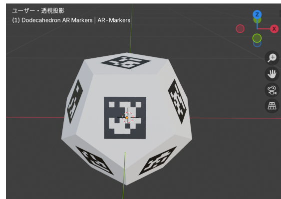
Figure 1. A 12-faced dodecahedron with ArUco markers affixed to its surfaces for pose estimation.
