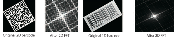
Figure4: 2D FFT of 2D and 1D barcodes.
