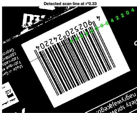
Figure7: Decode along scanline from both sides
