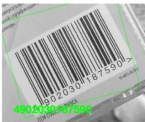
Figure11: Bounding box detected by morphological transformation
