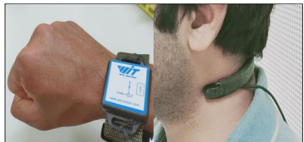
Figure I: Installation of IMU sensor on wrist position (left) and microphone on under the Ear Position (Right)
