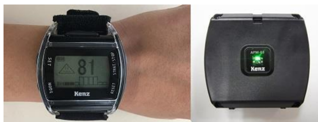
Fig1. Wristwatch-type pulse wave sensor with built-in 3-axis accelerometer.
