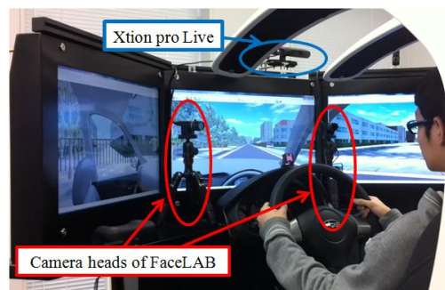
Fig. 2 Experimental system for measuring driver's behaviors.
