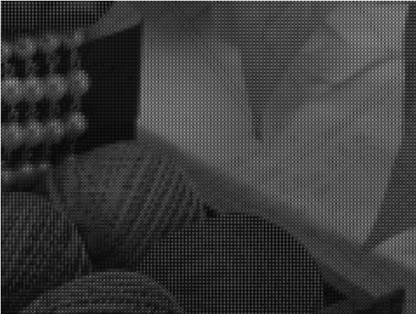
図 3: Magnified part of an image with embedded overlay information on emulated four color display
