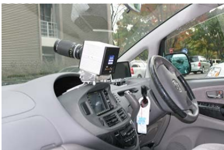
Fig. 4. High-speed camera used as receiver
