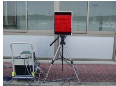
Fig. 3. LED array used as transmitter
