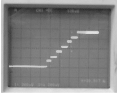
Figure 4: This waveform is an output state on 3-bit HNN quantizer. As an input signal, triangular wave is used. Its frequency is 10Hz and its amplitude is \pm 15 voltage.
