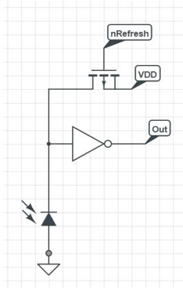
The basic photodiode circuitry is shown above. The Refresh signal is connected to the gate of the transistor. The source of the transistor is connected to VDD and the drain is connected to the photodiode whose other end is grounded.
