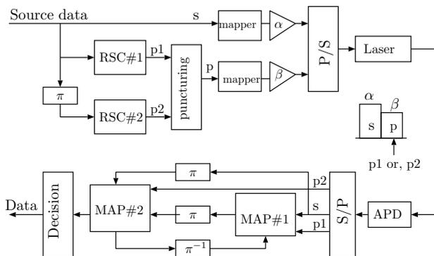
Fig. 1 System structure
