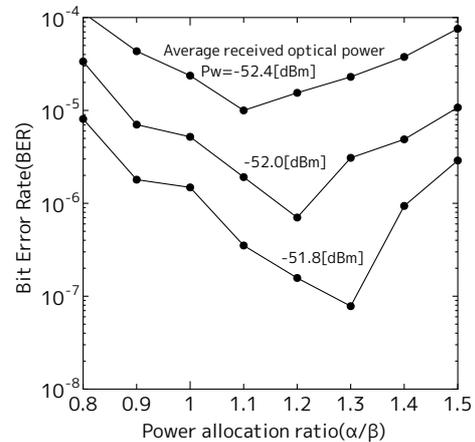
Fig. 2 BER vs transmission power allocation ratio
