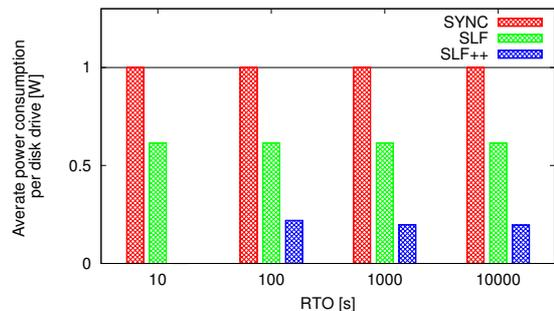
(a) Power reduction effect on IBM Ultrastar 36ZX
