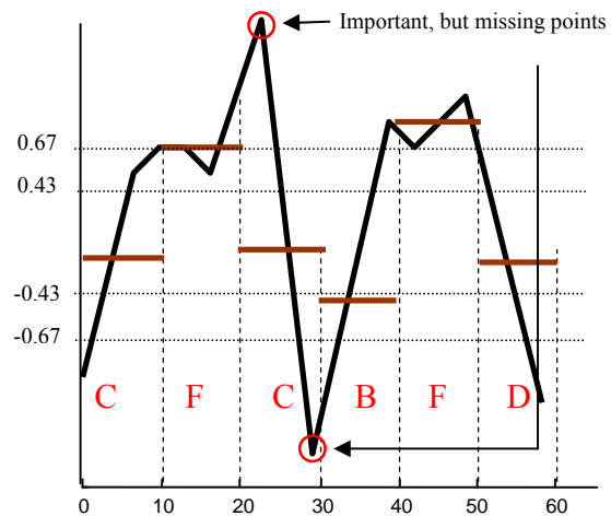
Figure 3: Financial time series data is represented by SAX. Some important points (shown in red) are missing. (US$ and Japanese yen exchange rate data of 2 months.) The SAX representation is CFCBFD .
