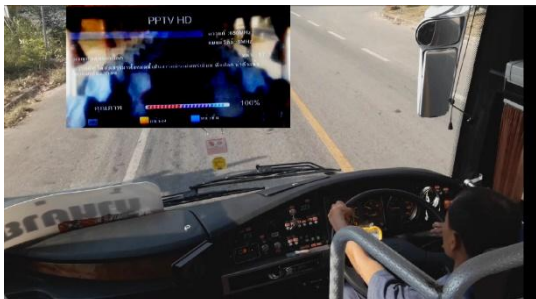
Fig. 5. Signal indicator on the screen showing strong received signal level while the bus was moving at the speed of 80 km/hr.
